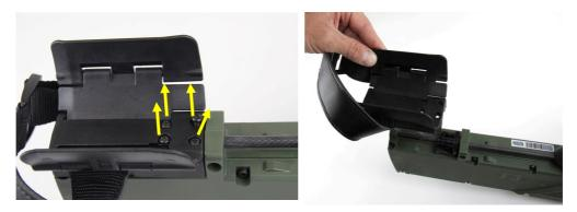
Figure 9: Removing the Armrest
