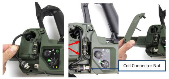
*Figure 70: Connecting Coil Cable and Cover*
