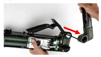
Figure 15: Removing Shafts
