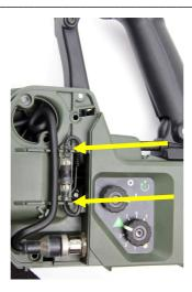
Figure 85: Correct Position of Wiring Loom Handle
