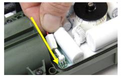
Figure 45: Connecting Battery Connector
