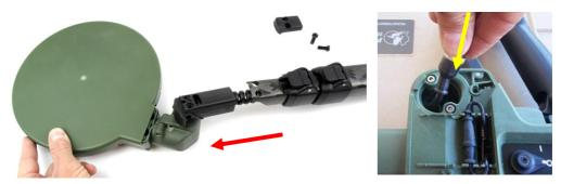
*Figure 53: Sliding the Coil Off the Shaft*
