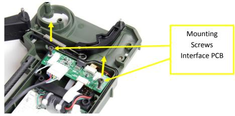
*Figure 34: Interface PCB*
