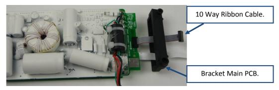
Figure 38: Fitting Bracket
