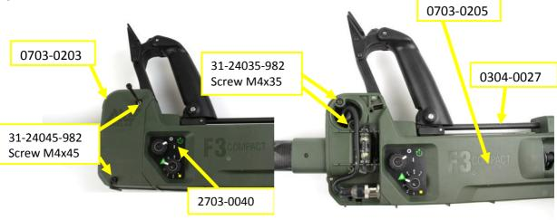
Figure 100: Detector left side
