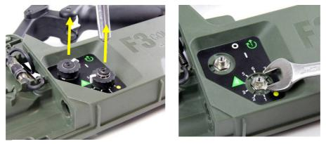
Figure 93: Removing Control Switch Knobs
