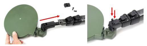
Figure 68: Fitting Coil to Lower Shaft
