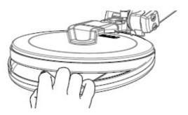
*Figure 48: Replacing the Skid Plate*
