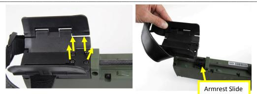
Figure 87: Removing the Armrest
