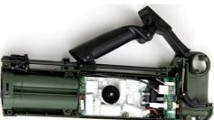
Figure 89: Opened Detector Body
