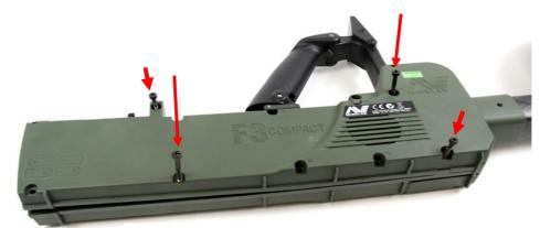
Figure 22: Fitting Four Screws
