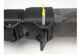
Figure 73: Fitting Camlock Pin
