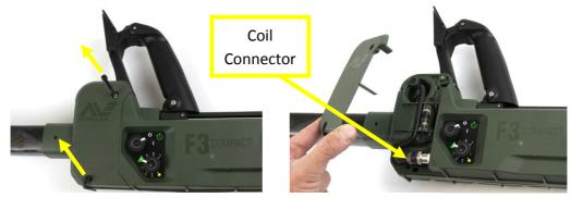
Figure 49: Removing Hinge Cover
