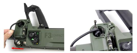
Figure 11: Disconnecting Coil Plug and Removing Screws
