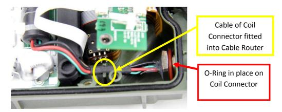
Figure 41: Coil Connector
