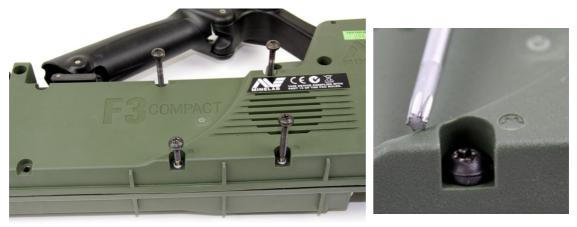
Figure 13: Removing Four Torx Screws
