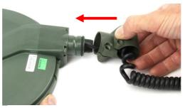
Figure 61: Fitting Pivot Coil Yoke
