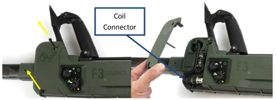
Figure 10: Removing Hinge Cover
