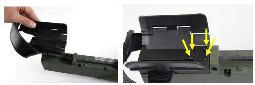
Figure 28: Attaching the Armrest
