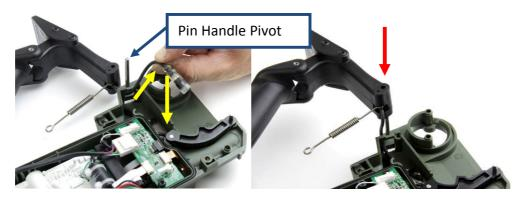
Figure 83: Threading the Wiring Loom
