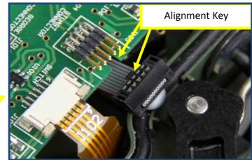
Figure 43: Connector 10 Way
