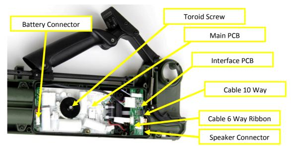
Figure 29: Detector Body and Main PCB
