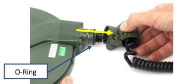
Figure 59: Removing Pivot Coil Yoke
