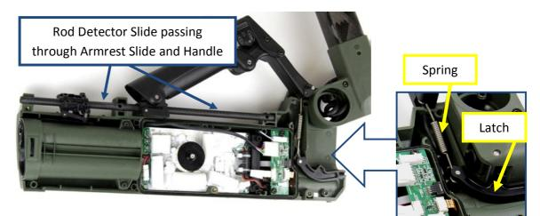
Figure 19: Latch Hinge and Spring Latch Hinge
