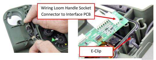
Figure 99: Wiring Loom Handle Socket
