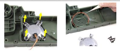
Figure 96: Replacing Speaker Assembly
