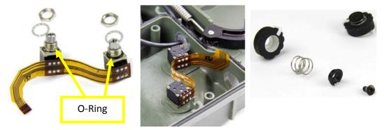
Figure 94: Control Switches
