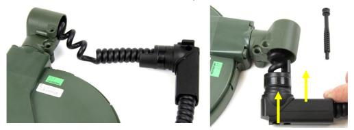
Figure 62: Fitting Pivot Lower Shaft
