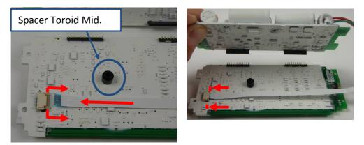
Figure 37: Connecting Six Way Ribbon Cable
