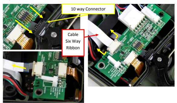
Figure 35: 10 Way Connector and Six Way Ribbon Cable
