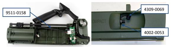
Figure 97: Wiring Loom Earset Kit
