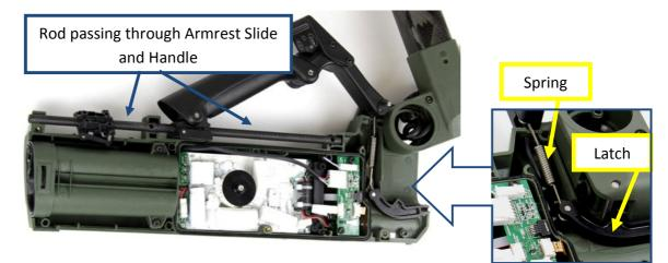
Figure 84: Latch Hinge and Spring Latch Hinge
