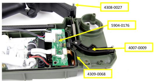
Figure 103: Detector body
