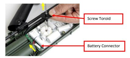
Figure 33: Screw Toroid & Battery Connector
