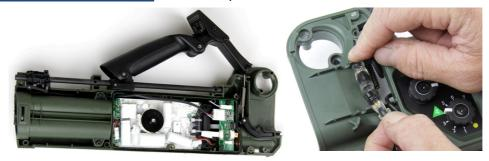
Figure 80: Disconnect Wiring Loom Handle
