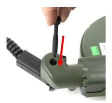
Figure 63: Inserting Pin Coil Pivot
