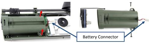
Figure 90: Replacing Battery Compartment
