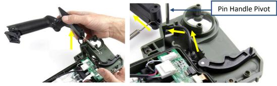
*Figure 82: Removing Handle and Cable*
