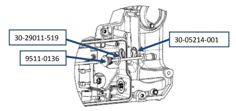
Figure 98: Wiring Loom Handle Socket Kit
