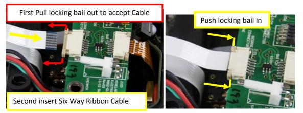
Figure 44: Connecting Six Way Ribbon Cable
