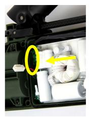
Figure 40: Fitting Main PCB
