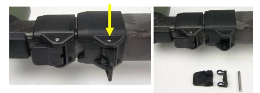
Figure 72: Removing Camlock Pin
