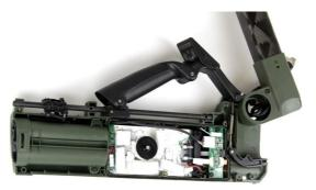
Figure 69: Fitting Shaft and Coil
