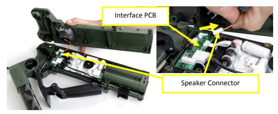
Figure 14: Disconnecting Speaker Connector
