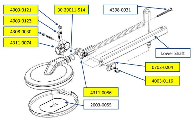
Figure 47: Parts of the Coil
