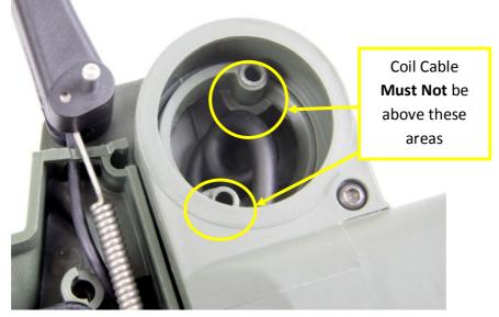
Figure 21: Coil Cable Position in Shaft Hinge
