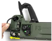
Figure 50: Disconnecting Coil Connector
