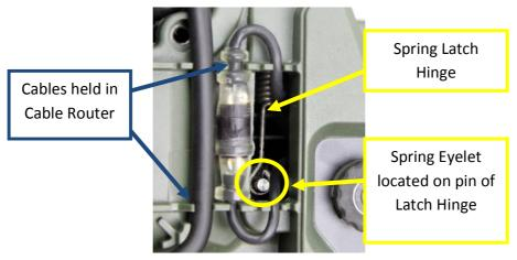
Figure 26: Underneath Hinge Cover
