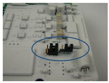
Figure 39: Three Jumpers on Main PCB
