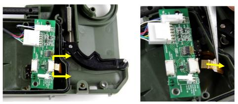
Figure 92: Disconnecting Six Way Ribbon Cable
