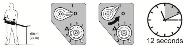
Figure 3: Switch On
